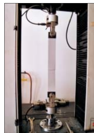
Spectraplan ® thermische las overlap. Naad sterker dan de dakbaan zelf.
